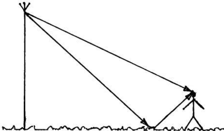
The total field at R is then the sum of the direct and reflected rays which can be written as  $E = E_d + E_r = E_d(1 + \Gamma)$ . Now power density  $S$  is proportional to  $E^2$ , hence the term  $(1 + \Gamma)^2$  must be included in the defining equations for power density. Thus
